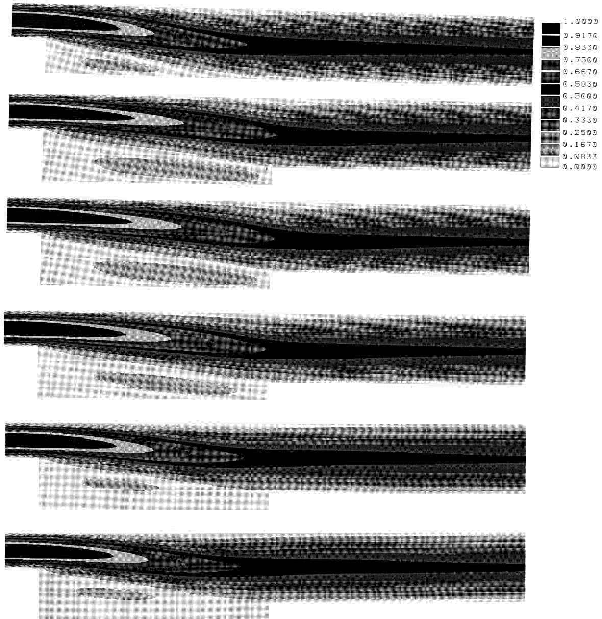
Fig. 8. Velocity contours for porous segments with different pressure loss coefficients. From top: reference flow, KP = 10^{-2} , KP = 1.0 , KP = 10^2 and KP = 10^4 .
