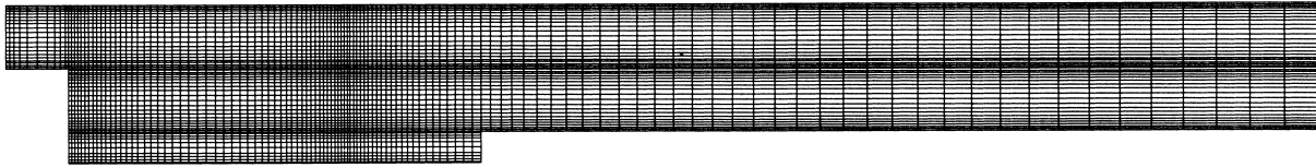
Fig. 2. Finite element mesh used for the case of L_p = 6.6 and D_p = 0.5 .
